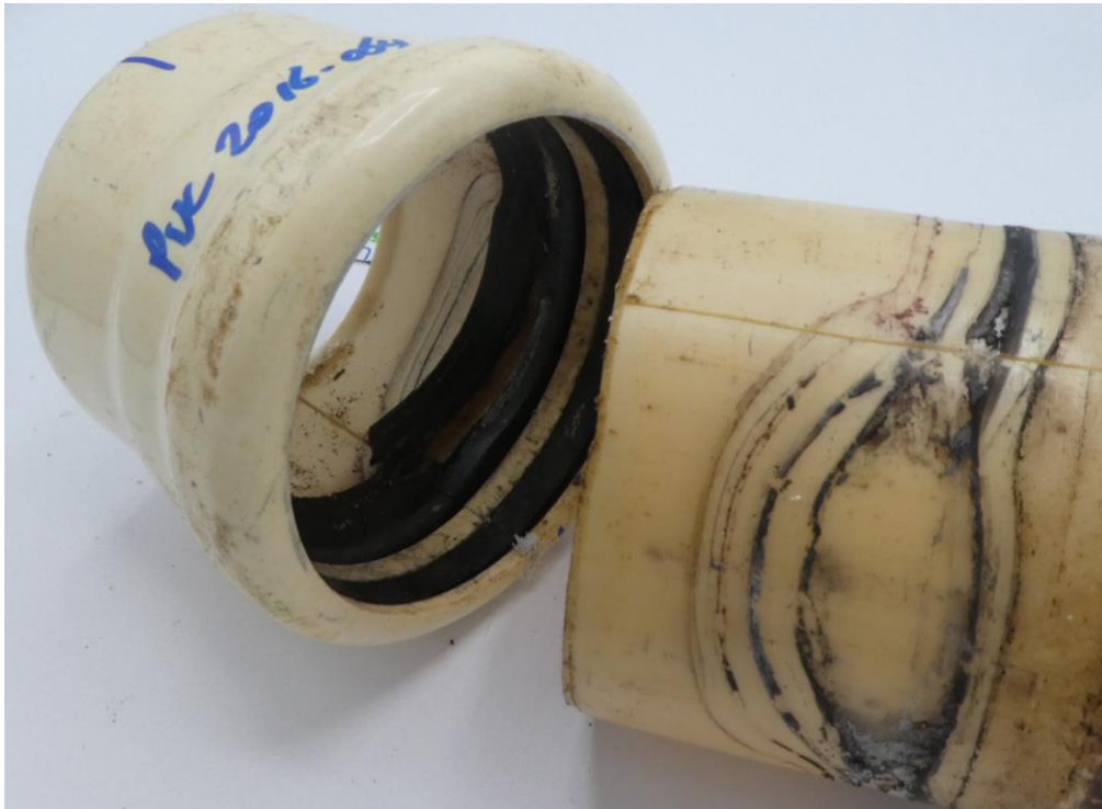
Figure 21 De-mounted joint PVC 2016-064 after testing
