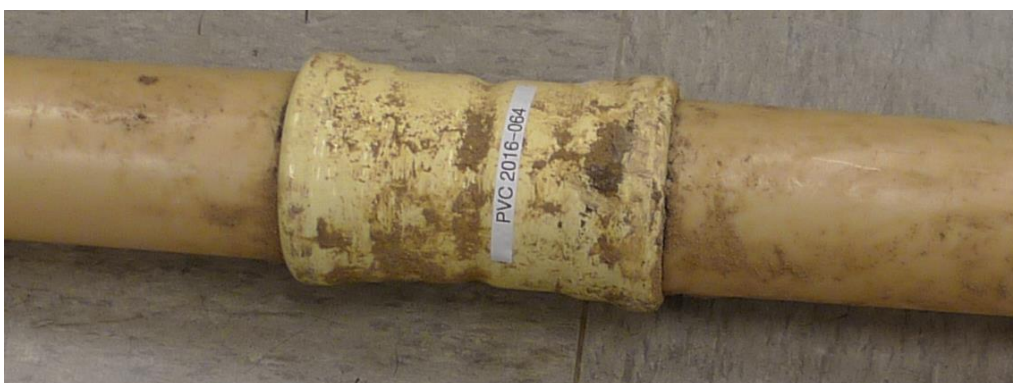
Figure 7 PVC 2016-064; PVC-U thermo formed coupler and PVC-U pipes
